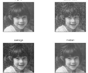
Fig 3: Effect of Median filtering on images
